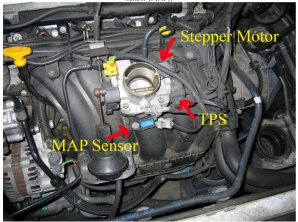
4. Unscrew the throttle body and remover the stepper motor:
