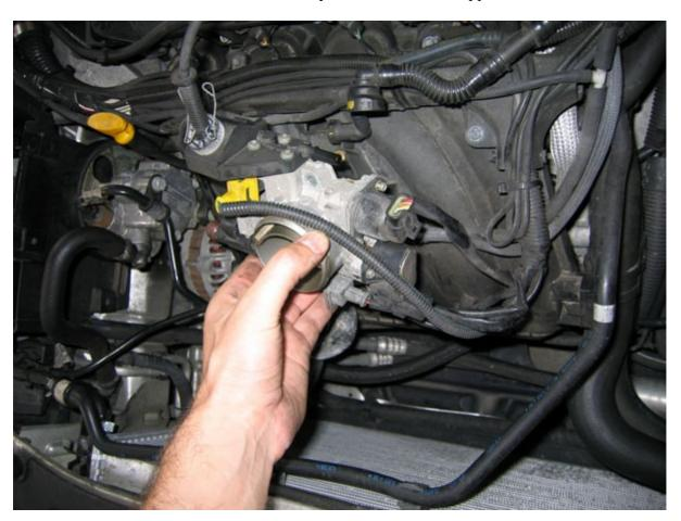
5. Clean the stepper motor with degreasing spray (brake cleaner) and put a little WD40 in for lubrification:
